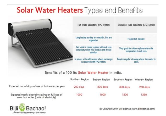
For this report, a 100-liter capacity solar water heater is considered. A 100-liter, EPC solar water require requires 20 square feet of space. The energy saving from the system is calculated a follow:
